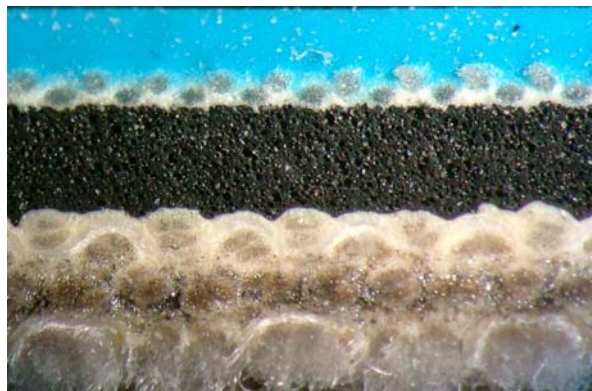
A typical compressive blanket with four plies. Please note the voids free structure and reinforcements almost vitreous look.
