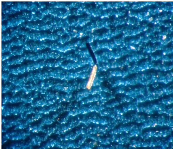
A blanket surface rubber with a catalyst crystal incrustation with 260 \times 40 \mu\text{m} after being easily removed from the elastomer surface and the respective hole.
