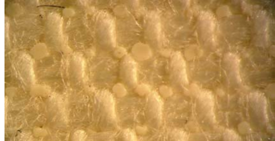
Carcass cloth surface showing rubber 'spots' from the first to the second ply gluing film. These spots are suggestive of reinforcement fibres being well impregnated by the rubber matrix.
